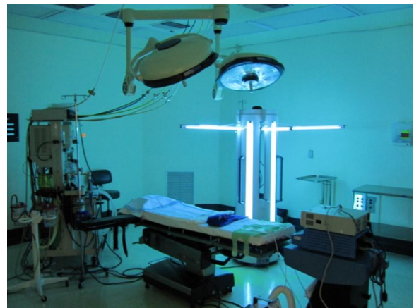
Figure 1. The Portable, Dual-Mode, Large-Area UVG Device shown closed (top photo) and operational in open mode (bottom photo).
